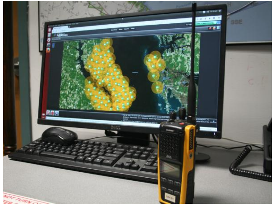
Improvement to hand held radios, such as longer antennae, have made the Harris system in use by the county more reliable.
