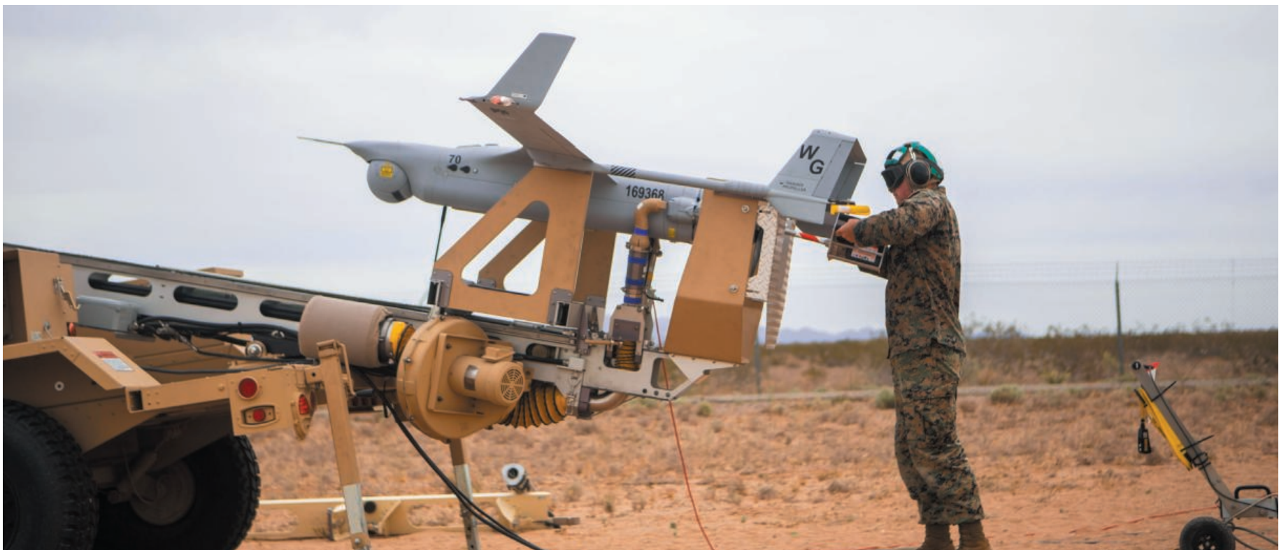
A U.S. Marine places the starter into an RQ-21A Blackjack during a recent Weapons and Tactics Instructor course at Canon Air Defense Complex in Yuma, Az. U.S. Marine Corp photo by Lance Cpl. Auburne Johnson)
