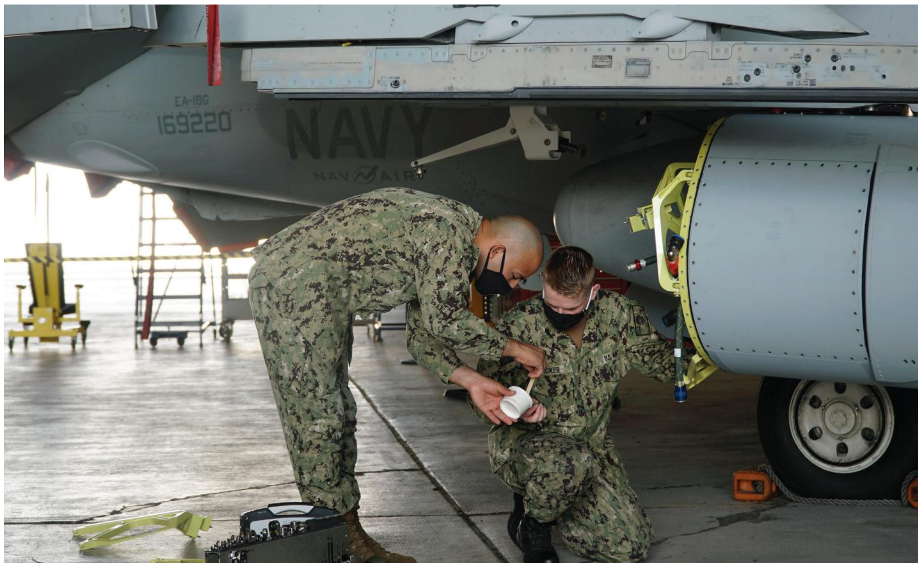
Aviation Electronics Technician 2nd Class Jean Fernandez and Aviation Electronics Technician Airman Michael Acker conduct maintenance procedures on the aft section of a Next Generation Jammer Mid-Band pod.
