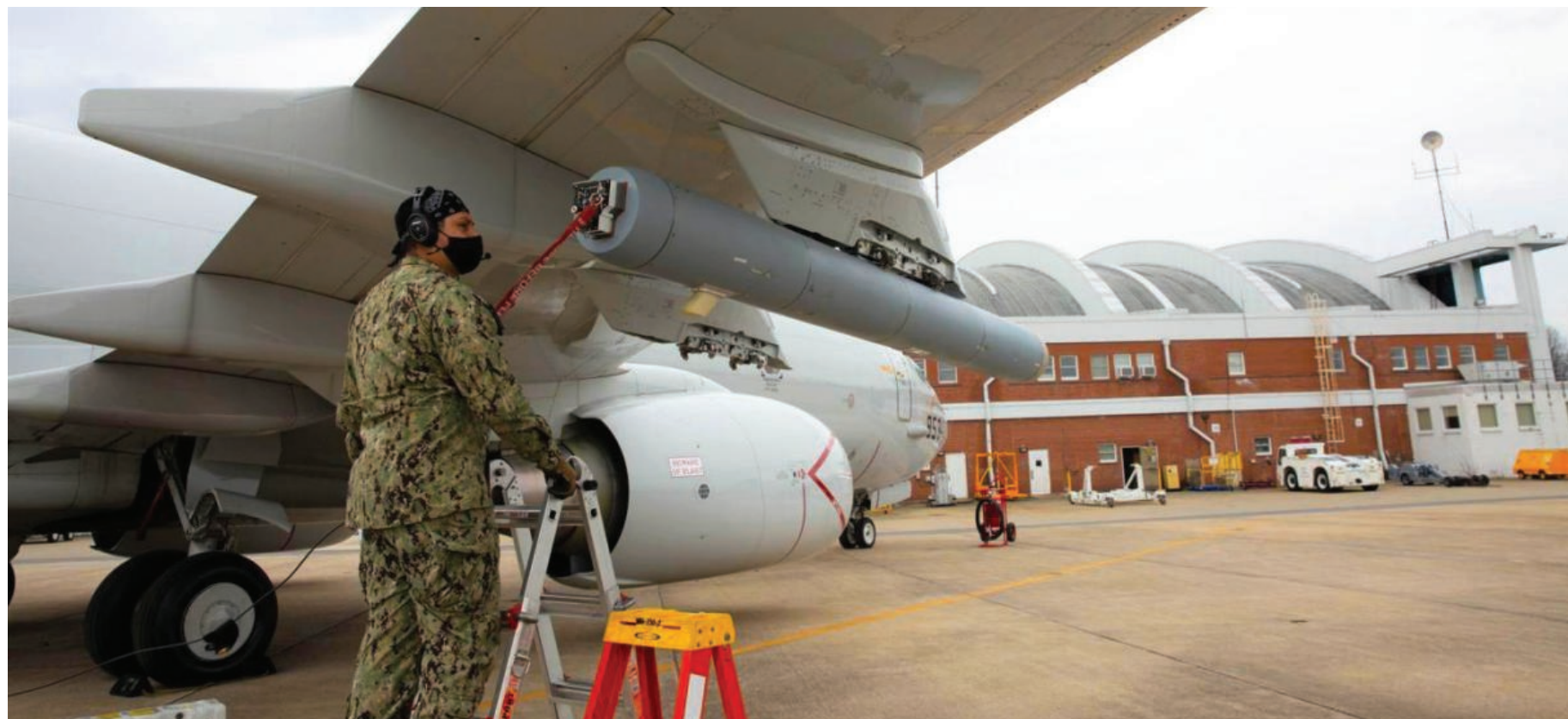
A member of Air Test and Evaluation Squadron (VX) 20 puts a pod-mounted radio frequency countermeasure system on a P-8A Poseidon, March 12. The pod successfully completed an air worthiness test at the Naval Air Warfare Center Aircraft Division (NAWCAD) Atlantic Test Ranges at NAS Patuxent River
