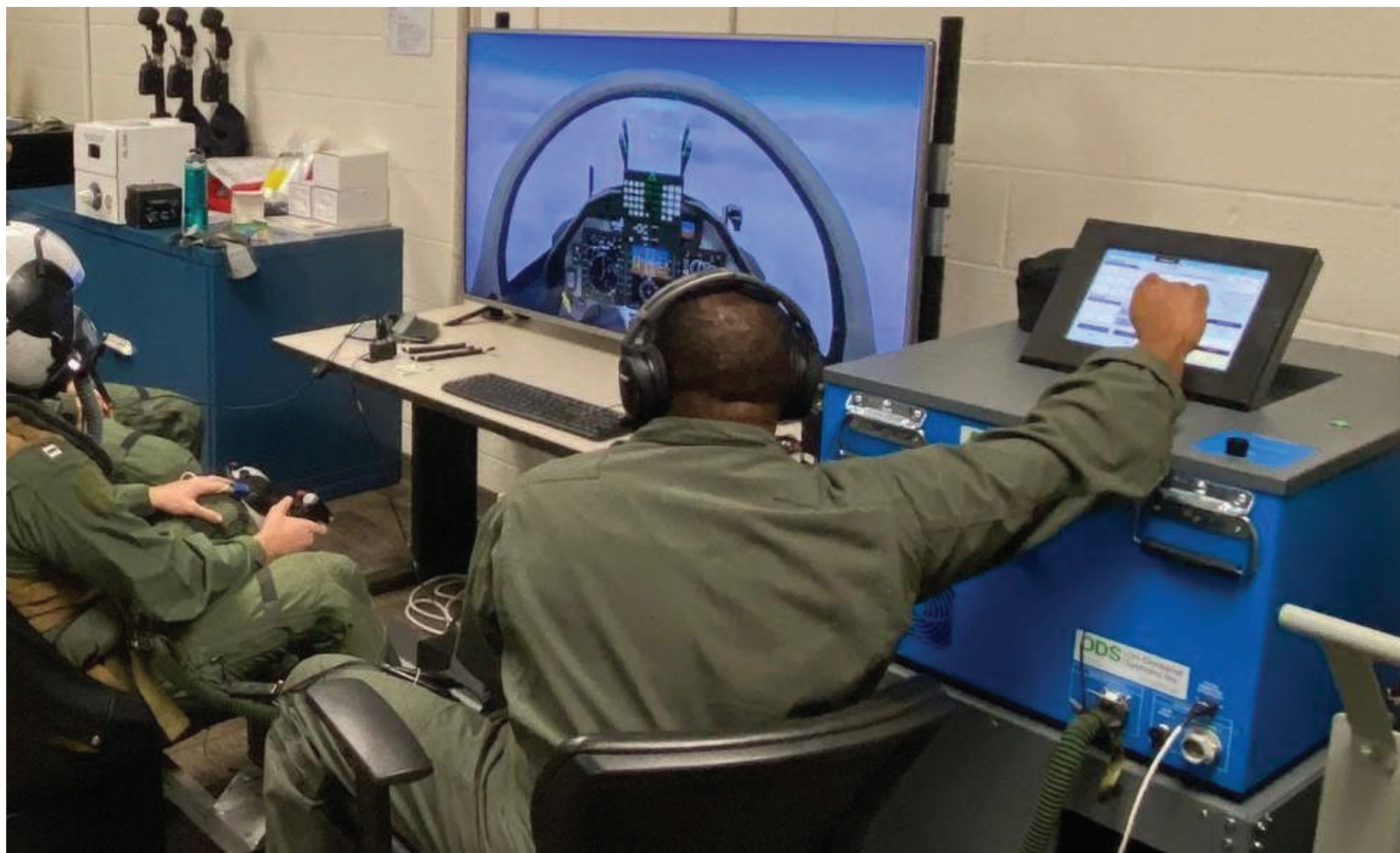
Navy Hospital Corpsman first class Marcus K. Billingsley provides training on the newly installed Mask on Breathing Device (MOBD) at the Aviation Survival Training Center, Pensacola, Fla. (U.S. Navy photo)
