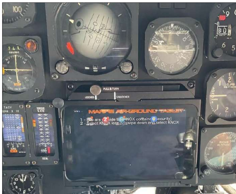
The Mission Data Extender (MDE) is a fully integrated, hard-mounted commercial off-the-shelf tablet which functions as a primary mission display in the CH-53E Super Stallion helicopter cockpit.
