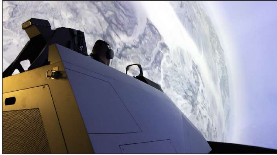
A pilot tests a U.S. Air Force F-22 Raptor cockpit simulator headed for installation in the Naval Air Warfare Center Aircraft Division's Joint Simulation Environment.
