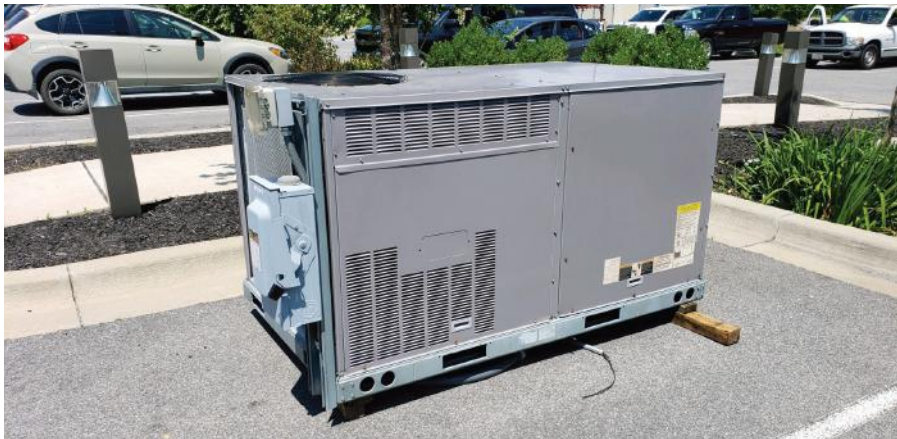
Mote Management Company donated this commercial, package/roof top, heat pump/air conditioning HVAC unit with an economizer and controls to CSM students for training.
