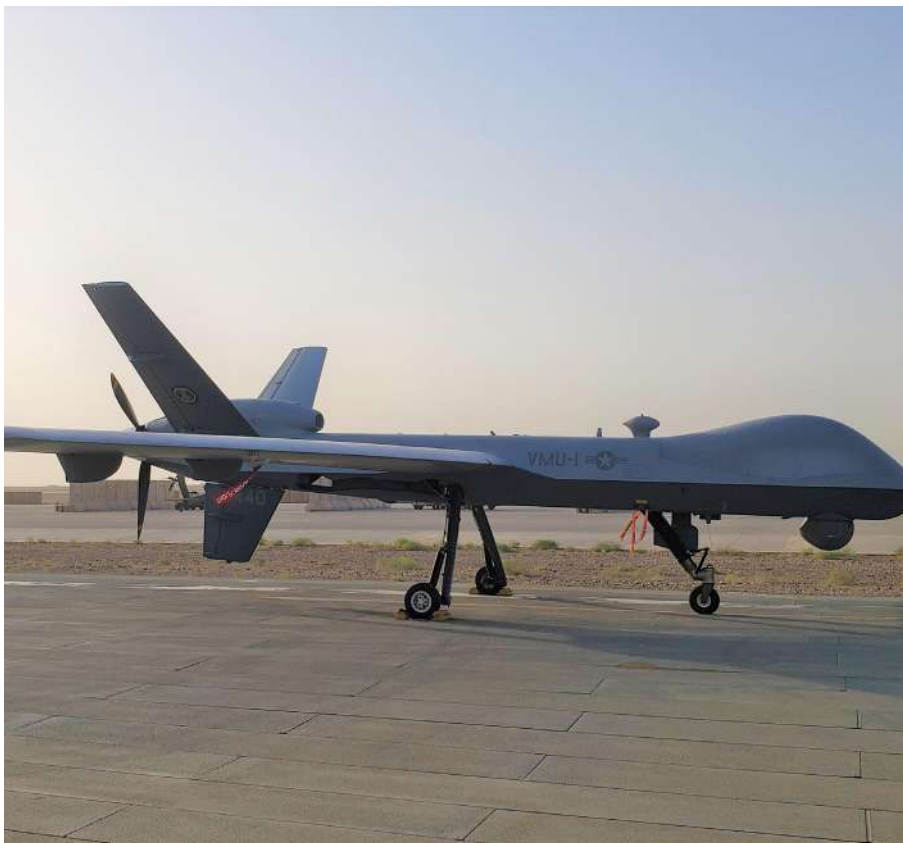
The MQ-9 Reaper provides Marines with a long-range intelligence, surveillance, and reconnaissance capability in support of expeditionary advanced based operations, littoral operations in contested environments, and maritime domain awareness. (U.S. Marine Corps photo)
