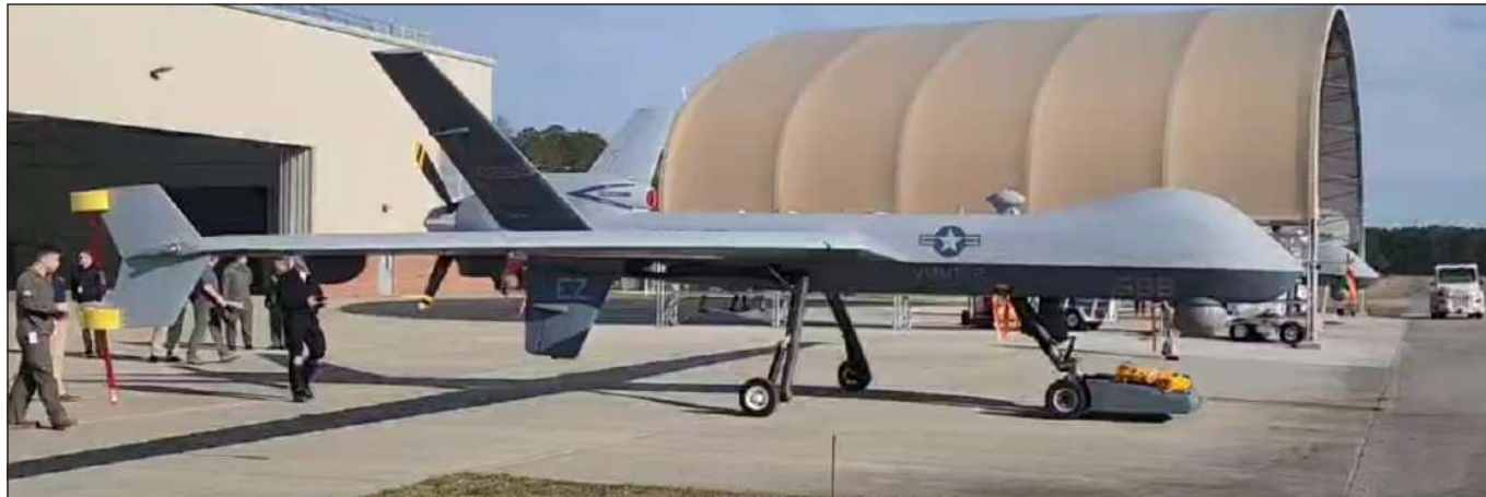
Marines test the TowFLEXX TF-3 Milspec, a new aircraft tug capability, with the MQ-9A Reaper at Marine Corps Air Station Cherry Point in March 2025. The TowFLEXX allows a single operator to maneuver military aircraft with unprecedented precision, maintaining the aircraft's nose wheel alignment while enabling 360-degree turns in confined spaces. (U.S. Navy photo)
