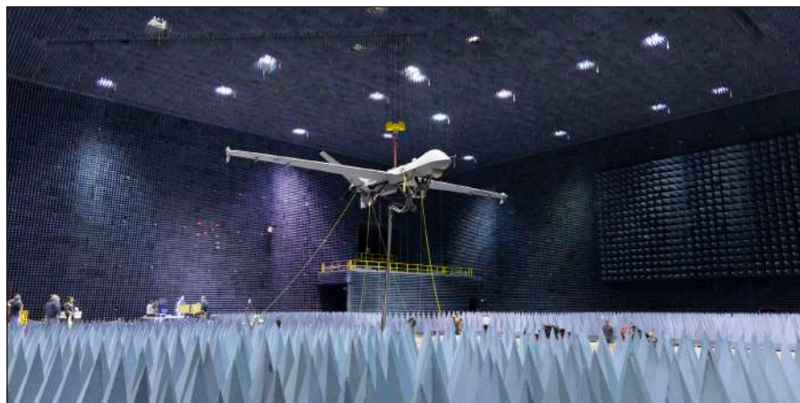
A Marine Corps MQ-9A Reaper undergoes anechoic chamber testing Feb. 24 at Naval Air Station Patuxent River, Md. (U.S. Navy photo)
