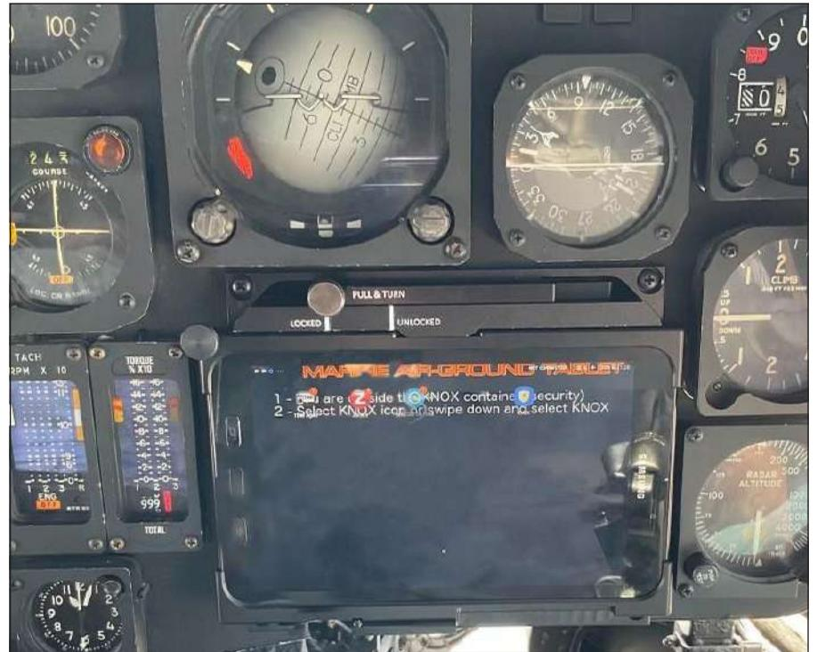
The Mission Data Extender (MDE) is a fully integrated, hard-mounted commercial off-the-shelf tablet which functions as a primary mission display in the CH-53E Super Stallion helicopter cockpit.
