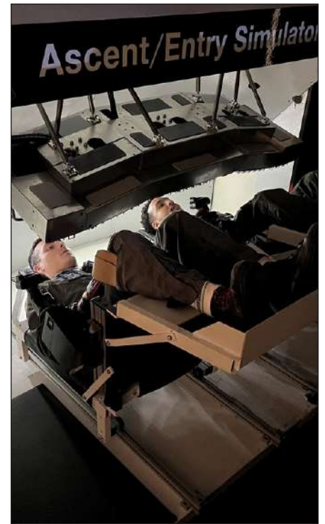
U.S. Naval Test Pilot School students Lt. Nathaniel Kruder and Lt. Guy Williams evaluate the human-machine interface of the Orion spacecraft for NASA. (U.S. Navy photo)
