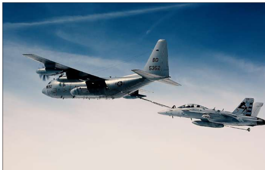
A U.S. Navy Reserve KC-130T refuels an EA-18G Growler in the skies over Naval Air Station Patuxent River in Maryland during testing that enabled the service's fleet of Hercules aircraft to aurally refuel a significantly expanded number of aircraft in early 2025.
