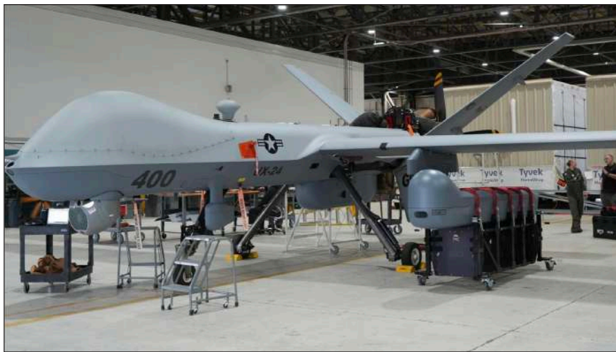
An MQ-9 Reaper is upgraded with SkyTower II Pod that will be deployed to Marine Corps' squadron next year to enhance operational capability. (U.S. Navy photo)
