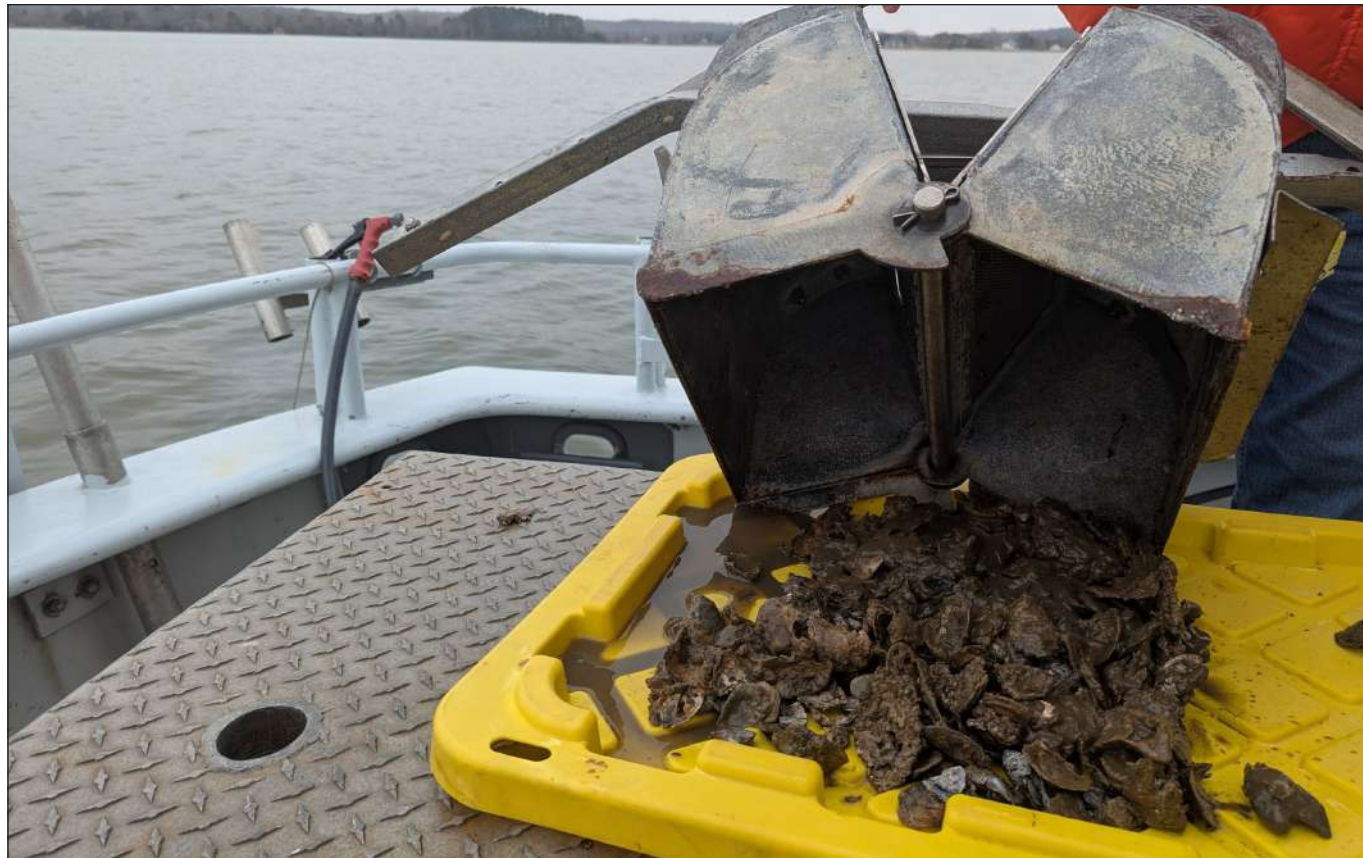
For ground truthing, or confirming their readings with material observations, the team pulls up samples and analyze the quality of the bottom, whether it's mud or soft sand—or filled with oyster shells. The team sometimes also uses an underwater camera to look at areas of the bottom. Photo by Joe Zimmermann/DNR
