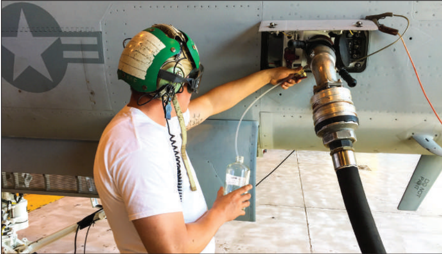
As part of test protocol, Aaron Williams, with Air Test and Evaluation Squadron (VX) 23 maintenance department, siphons a sample of the 100-percent alternative biofuel during ground test Aug. 30 at Naval Air Warfare Center Aircraft Division's Aircraft Test and Evaluation Facility. (U.S. Navy photos by Dan Owens)
