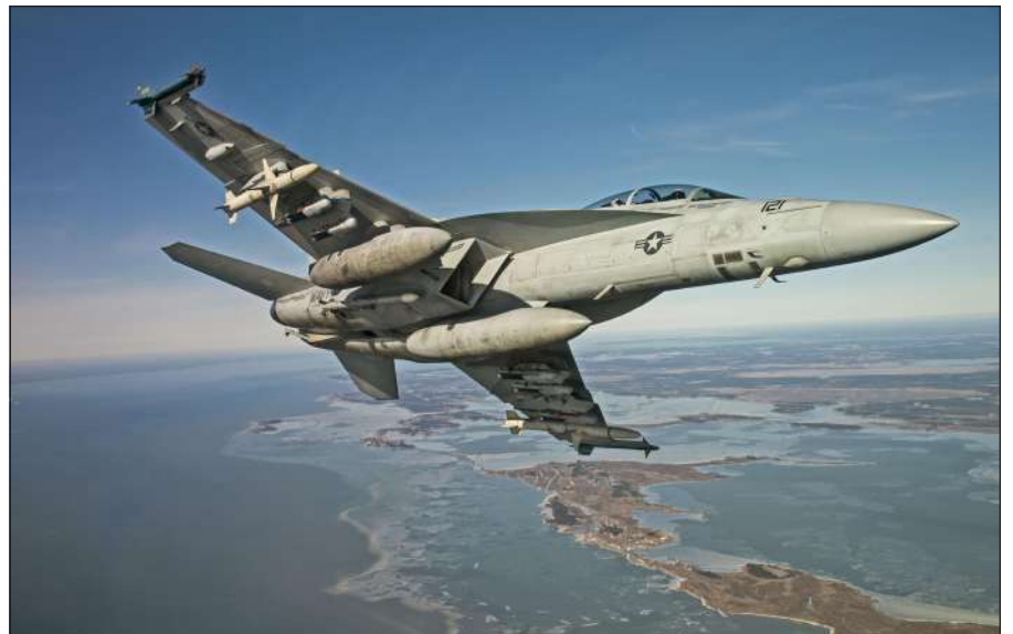
An F/A-18 conducts testing with the Small Diameter Bomb (SDB) II at Naval Air Station Patuxent River, Md. The SDB II variant includes an advanced tri-mode seeker, allowing it to engage dynamic targets in adverse conditions. (U.S. Navy photo)
